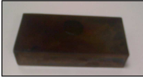
Fig. 3: Image of a flat-well polished carbon coated sample to be used for SEM imaging.
